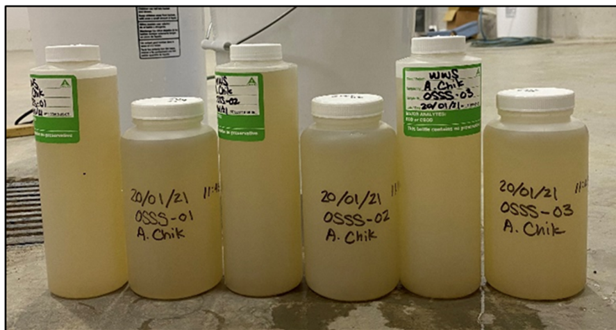
Figure S1. Visual check of wastewater aliquots obtained using the sample-splitting apparatus
