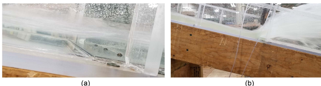
Fig. 4. Flow over spillway offsets: (a) attached to the flume floor at a small offset; and (b) detached from the floor at a large offset.
