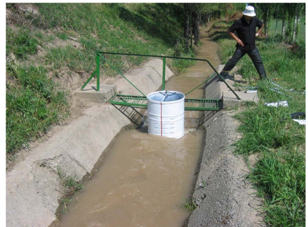
Fig. 6. Trapezoidal flume in use in Dushanbeh, Tajikistan (image by author)
