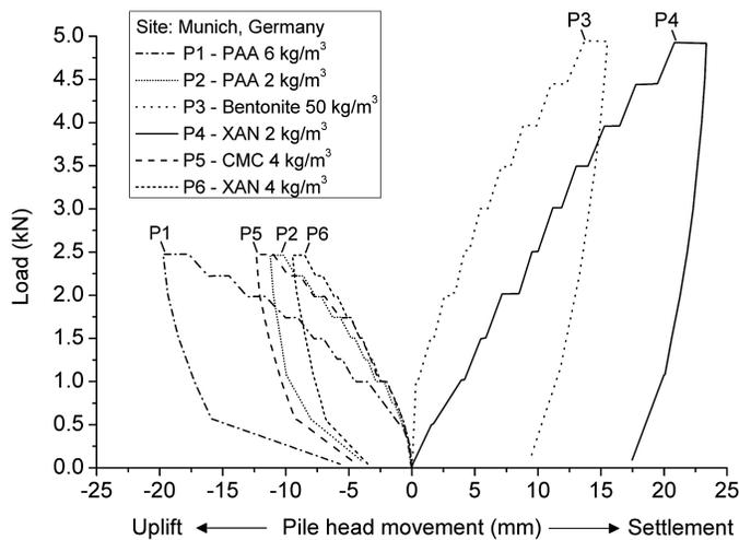
**Fig. 10.** Load–movement of six test piles constructed using bentonite and polymer fluids at Munich, Germany; intermediate unload–reload curves are removed for clarity (adapted from Lesemann 2010)
