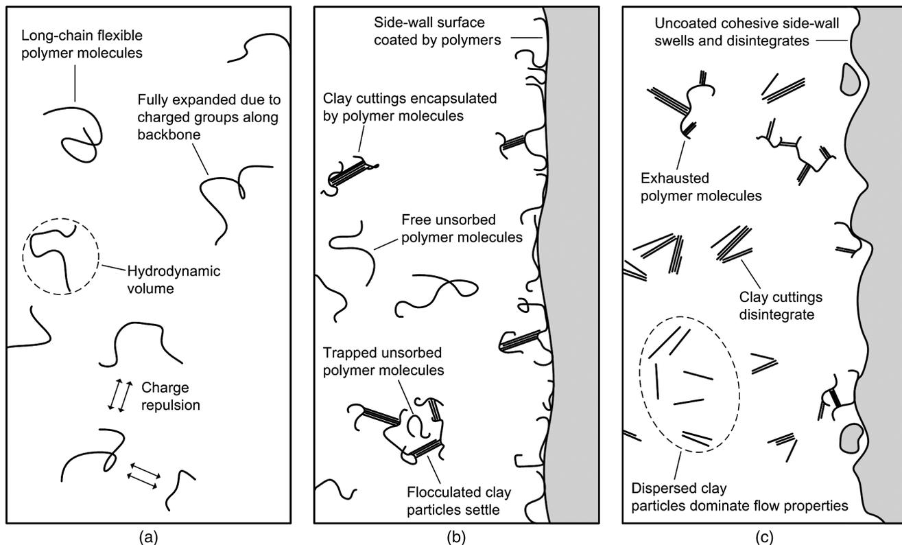
**Fig. 6.** Schematic interactions between polymer molecules and clay soil in an excavation supported by polymer fluids in different conditions (reprinted from Lam et al. 2014c, with permission; copyright ASTM International, 100 Barr Harbor Drive, West Conshohocken, PA 19428)
