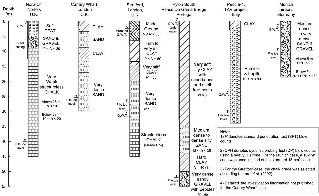
**Fig. 1.** Soil profiles, casing lengths, and pile toe levels at five European test sites
