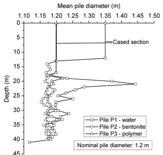
**Fig. 2.** Side-wall profiles of three test piles constructed using water, bentonite, and polymer support fluids at Norwich, United Kingdom (modified from Corbet et al. 1991)
