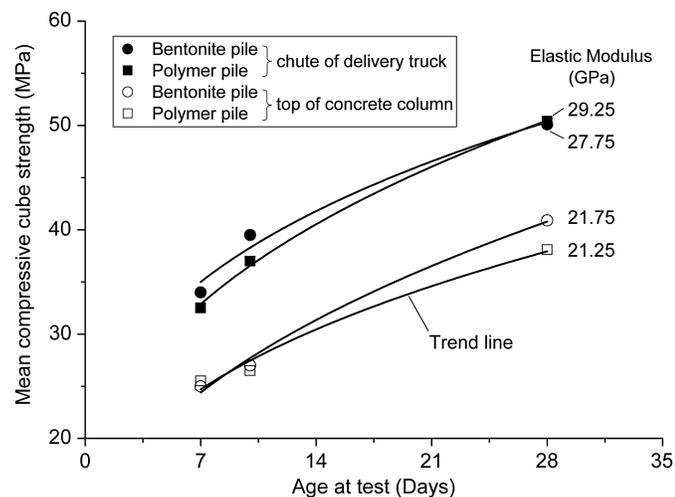
**Fig. 7.** Effect of bentonite and polymer support fluids on the compressive strength and stiffness of concrete (reprinted from Lam et al. 2010, with permission)
