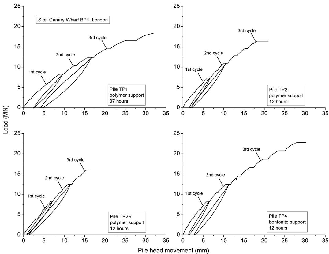
**Fig. 4.** Load–movement curves of four test piles constructed using bentonite and polymer support fluids at Canary Wharf in London, United Kingdom (data from D. Nicholson, personal communication, 2014)
