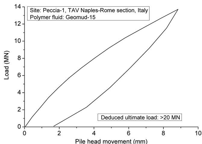
**Fig. 9.** Load–movement curve of a test pile constructed using polymer fluid at Peccia-1, Treno Alta Velocità project, Naples–Rome section, Italy (adapted from Bustamante et al. 1998)
