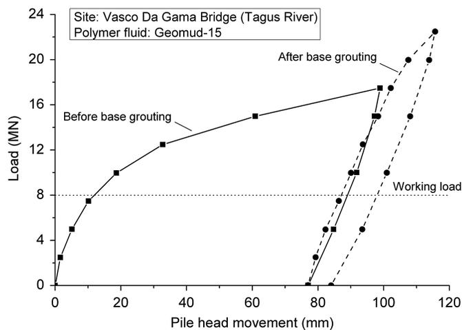
**Fig. 8.** Load–movement curve of a test pile constructed using polymer fluid at Pylon South, Vasco Da Gama Bridge, Portugal; intermediate unload–reload curves are removed for clarity (adapted from Guadagnini 2001)
