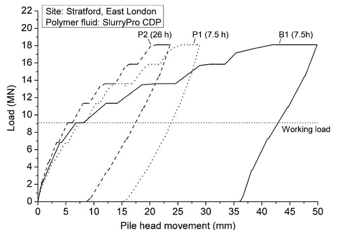
**Fig. 5.** Load–movement curves of three test piles constructed using bentonite and polymer fluids at Stratford, East London, United Kingdom; intermediate unload–reload curves are removed for clarity (adapted from Lam 2011)
