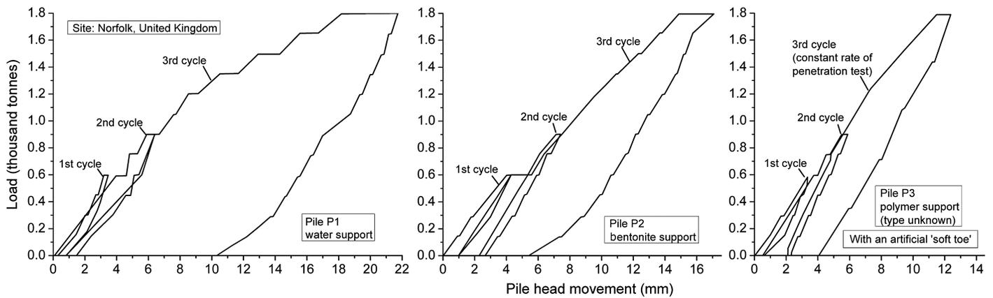
**Fig. 3.** Load–movement curves of three test piles constructed using water, bentonite, and polymer support fluids at Norwich, United Kingdom (modified from Corbet et al. 1991)
