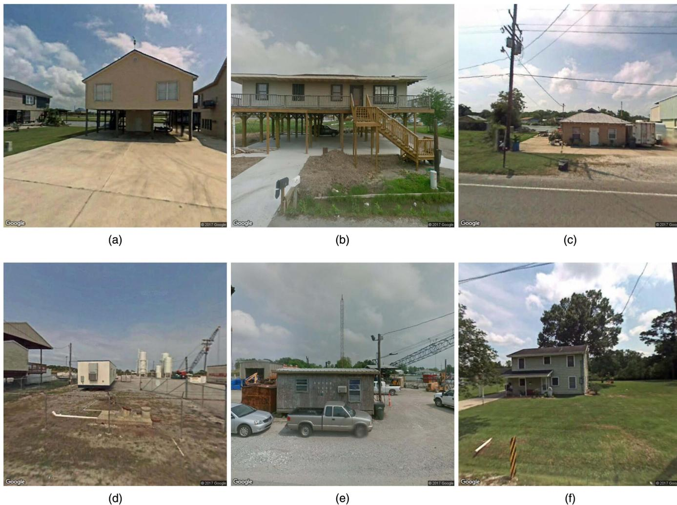
**Fig. 2.** Sample GSV images of typical buildings displaying: (a) high foundation heights; (b) pier foundations; (c) slab foundations; (d) mobile homes; (e) commercial buildings; and (f) two or more stories. (Images © 2017 Google.)
